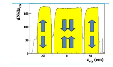
2 configurations: polarisation reversed each week to minimize possible systematic errors
