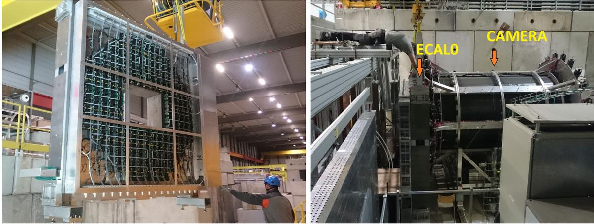
Figure 3.1: New detectors related to the second phase of the COMPASS experiment. *Left:* ECAL0 calorimeter during installation in the hall of the COMPASS experiment (March 2016). *Right:* A four-meter long recoil proton detector (CAMERA) and ECAL0 in final position (still unconnected to acquisition).
