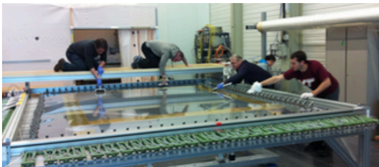
Figure 4.9: Stretching mylar on a cathode plane at CERN
