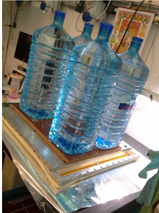
FIGURE 7.27: Application of pressure to ensure better gluing.
