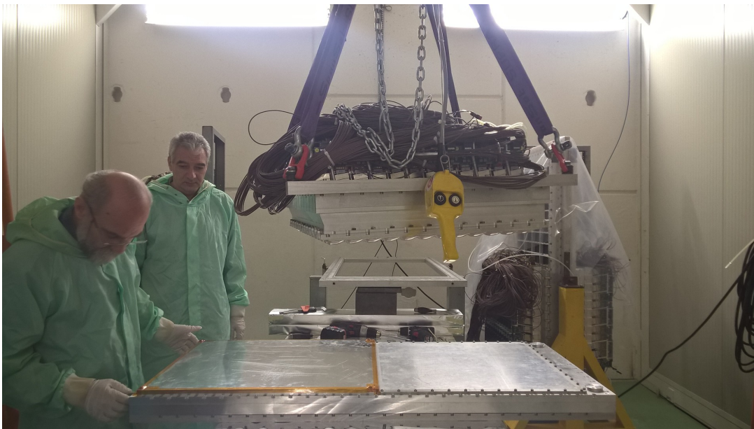
FIGURE 7.55: Mounting the MAPMTs with lenses to the new frame.
