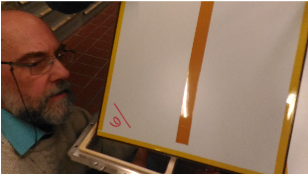
FIGURE 7.26: Attaching the PCB to the mechanical frame;
