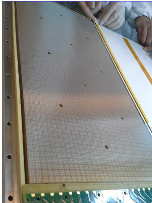
FIGURE 7.28: Stripping of the MicroMegas cover
