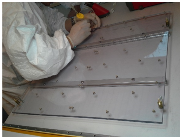
FIGURE 7.30: Mounting of PEEK pillars to the special frame
