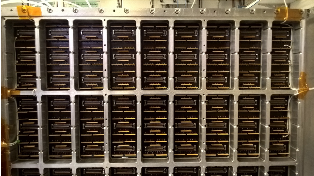
FIGURE 7.34: The Micromegas PCB (back view) after attaching the resistances;
