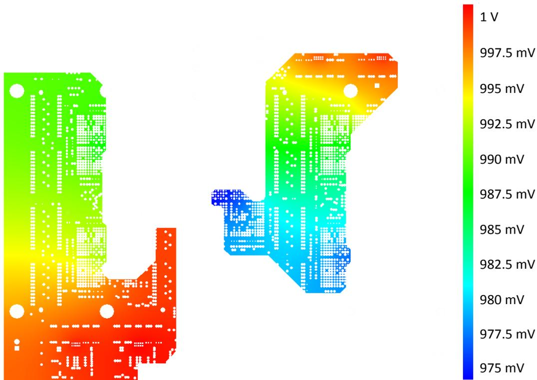
**Figure 4.25:** Simulation result for the voltage drop across the core supply planes. The deviation from the nominal voltage is below 2.6%.
