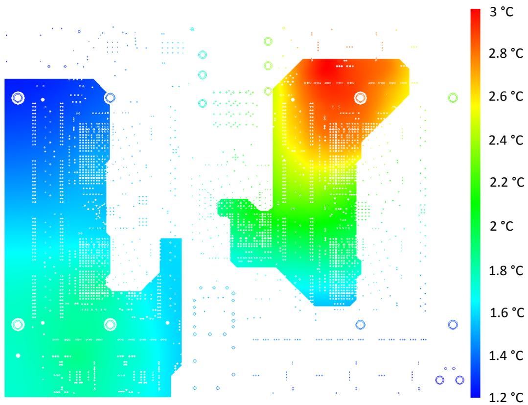
**Figure 4.26:** Simulation result for the temperature rise of the core supply planes due to joule heating.
