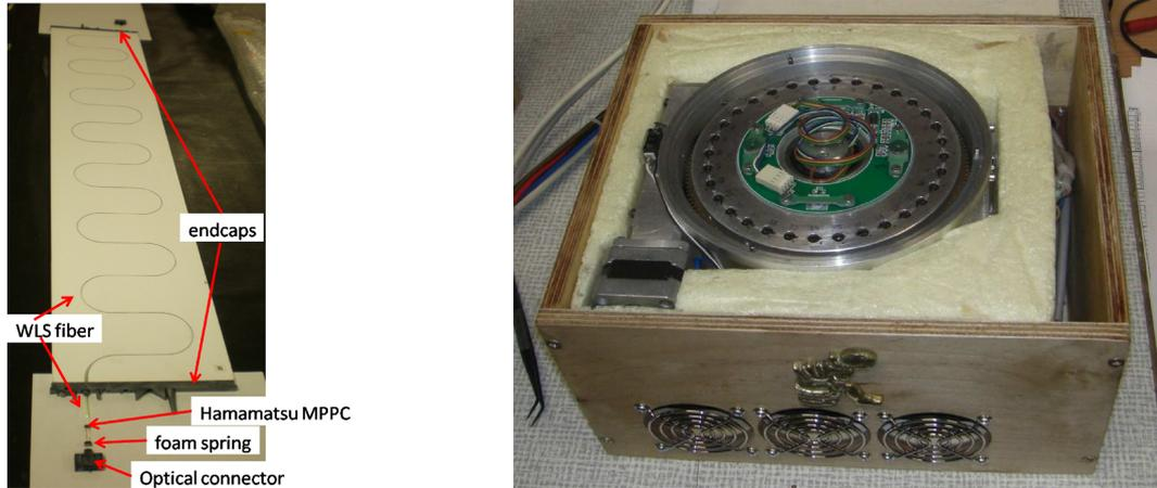
Figure 2.16: To the left: A single scintillator module of the SMRD detector - without a light-housing [32]. To the right: a part of automated system for measurement of MPPC detectors: the temperature stabilised feeder for 32 MPPC with preamplifier and LED flasher [34].
