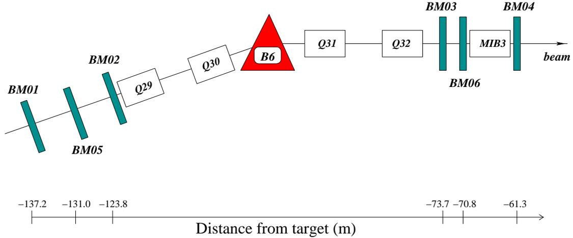
Figure 3.4: Layout of the BMS station [73].
