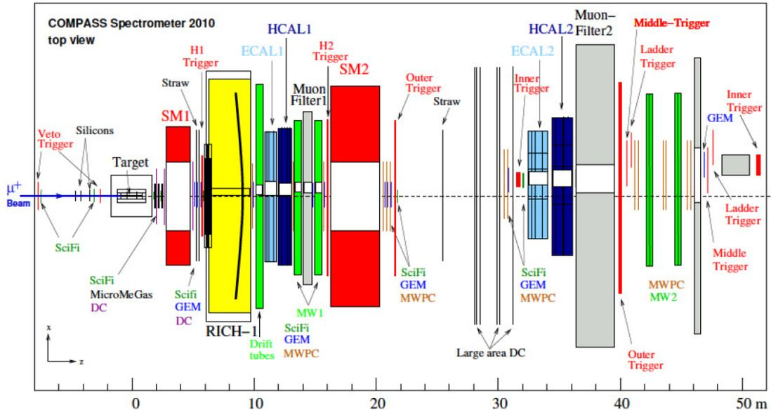
Figure 3.6: Top view of the COMPASS spectrometer in 2010 [83].
