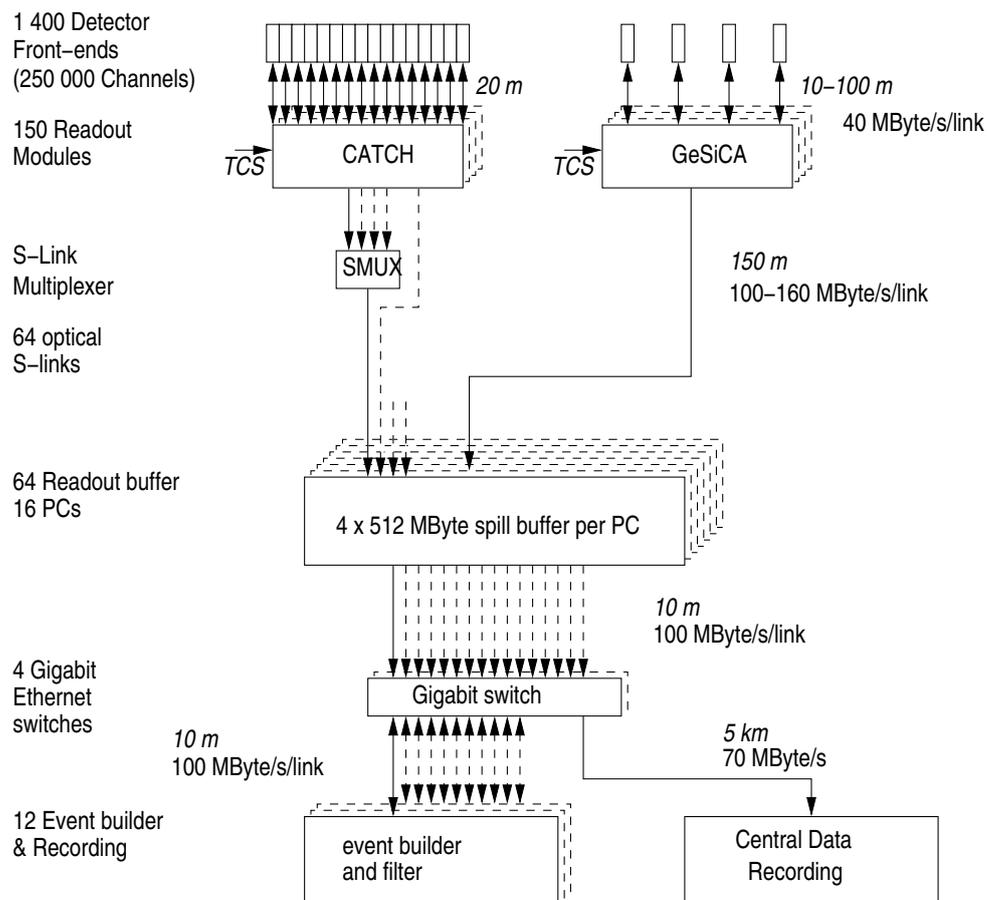
Figure 3.9: Architecture of the data acquisition [73].
