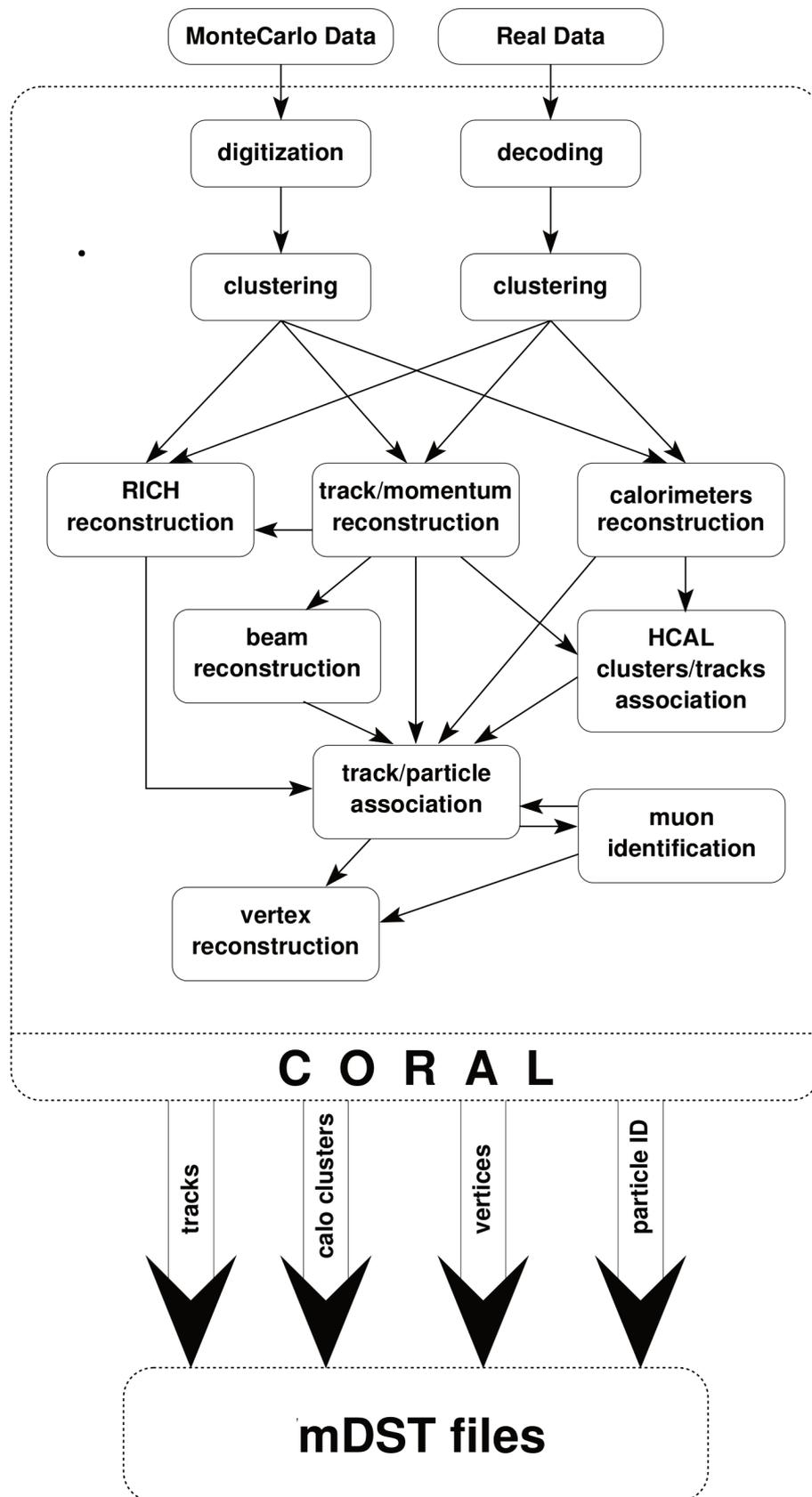
Figure 3.10: Reconstruction of data and MC [73].
