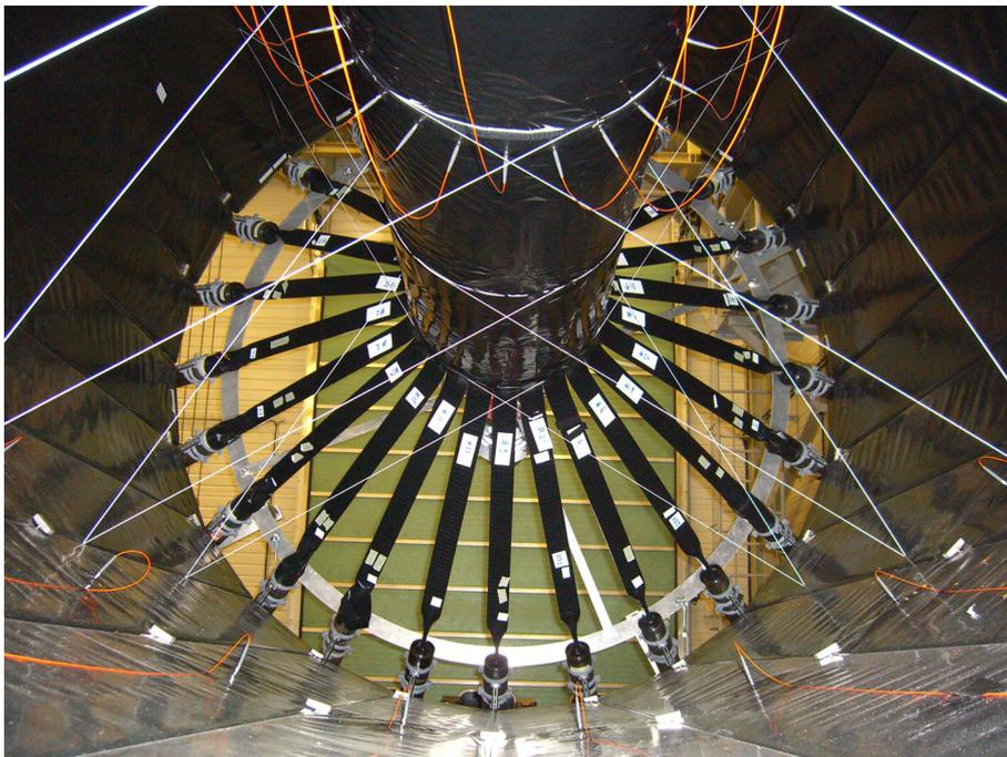
**Figure D.5:** View into the space between *Ring A* and *Ring B* of the CAMERA detector. The orange fibers are used for the laser calibration. *Ring A* is held in place by the white strings.
