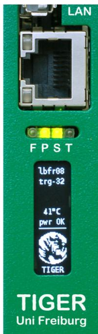
**Figure 5.34:** The TIGER module features four LEDs and an OLED display on its front panel. The meaning of the LEDs is explained in Tab. 5.17. The display is used to show general status information.
