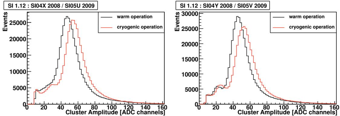
Figure 6.5: Cluster amplitudes for SI 1.12 for n-side (left) and p-side (right) for non-cryogenic (2008, black lines) and cryogenic (2009, red lines) operation. This detector module changed its place from SI04XY in 2008 to SI05UV in 2009.
