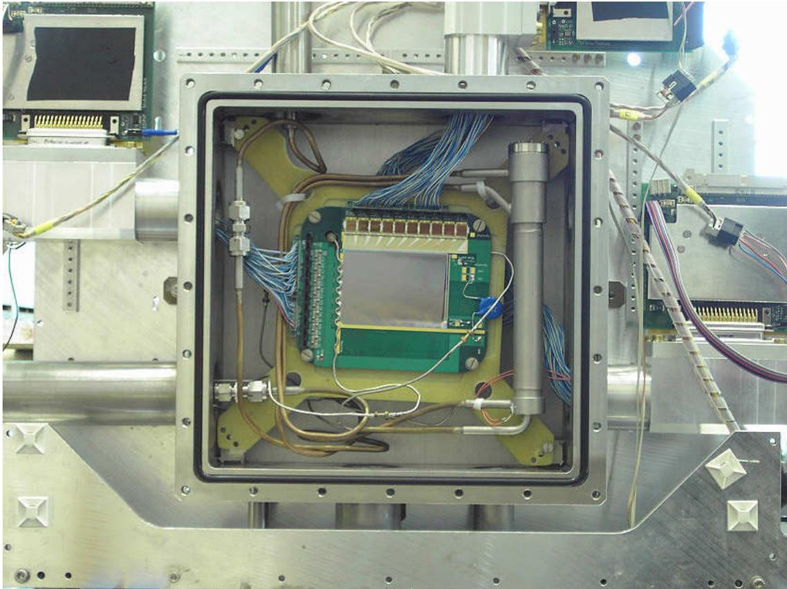
**Figure 4.7:** The first beam station cryostat, that was finally installed in the COMPASS area, in the lab. The *UV* detector module is visible, the *XY* module is mounted on the back side of the shuriken. The back window is substituted by a massive plate, which is exchanged with a beam window in the experimental area.
