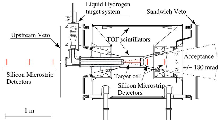
**Figure 3.8:** Scheme of the target region for 2008/9 and 2012 data taking, from [COM07a]. The beam enters from the left side. The silicon stations are indicated by vertical red lines; each line refers to the two modules of one station.
