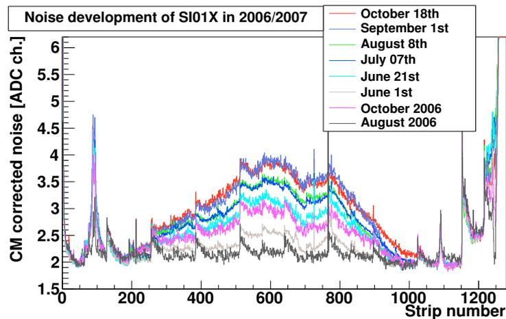
**Figure 5.4:** Noise development of the readout plane `SI01X` (from module `SIL10`) during 2007. For comparison also two curves obtained in 2006 are shown. The shadow of the beam profile is clearly visible as increased noise.
