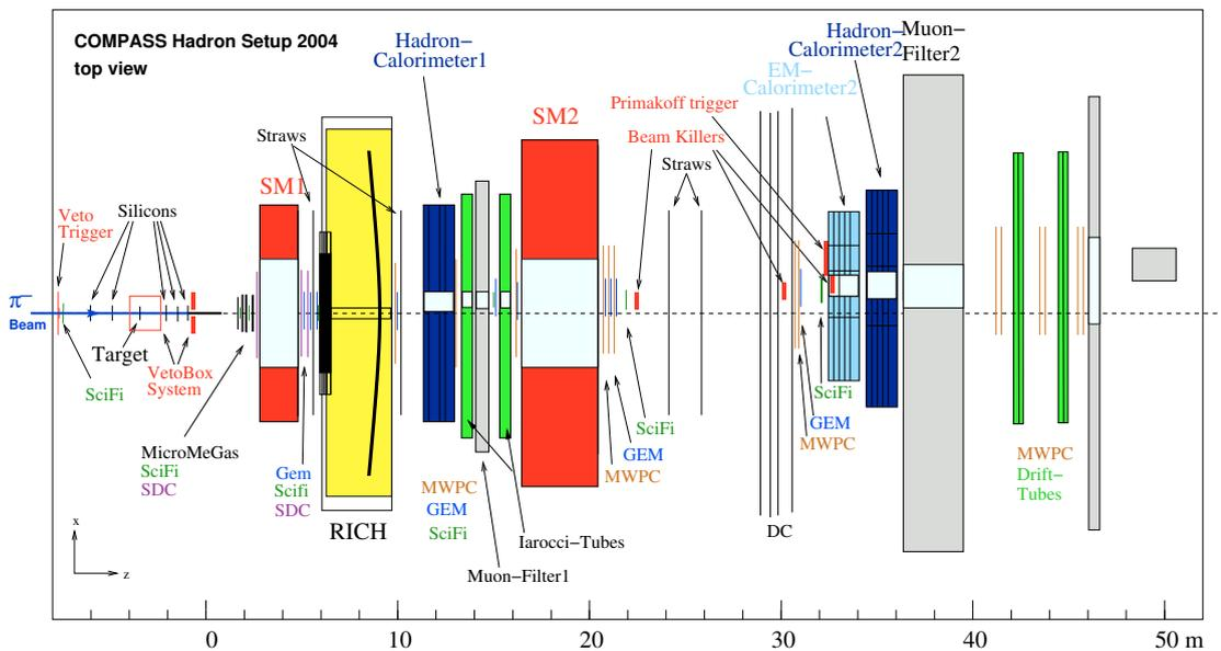
**Figure 2.3:** Sketch of the COMPASS spectrometer setup as used during the 2004 hadron run, from [COM].
