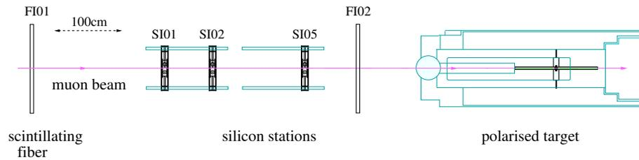
**Figure 3.5:** Silicon stations in the muon setup, with the specific names used in the 2004 muon setup, from [Din10]
