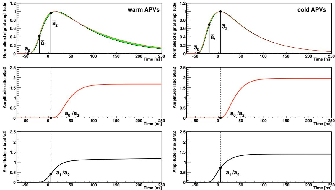
**Figure 6.2:** Comparison of the APV signals for warm (left) and cold (right) detectors, adapted from [Zim11]. The mean position of the samples is marked. For signal shapes as well as the single ratios, the red curve is constructed from the  $r_0$  and the black curve from the  $r_1$  time calibration parameters.
