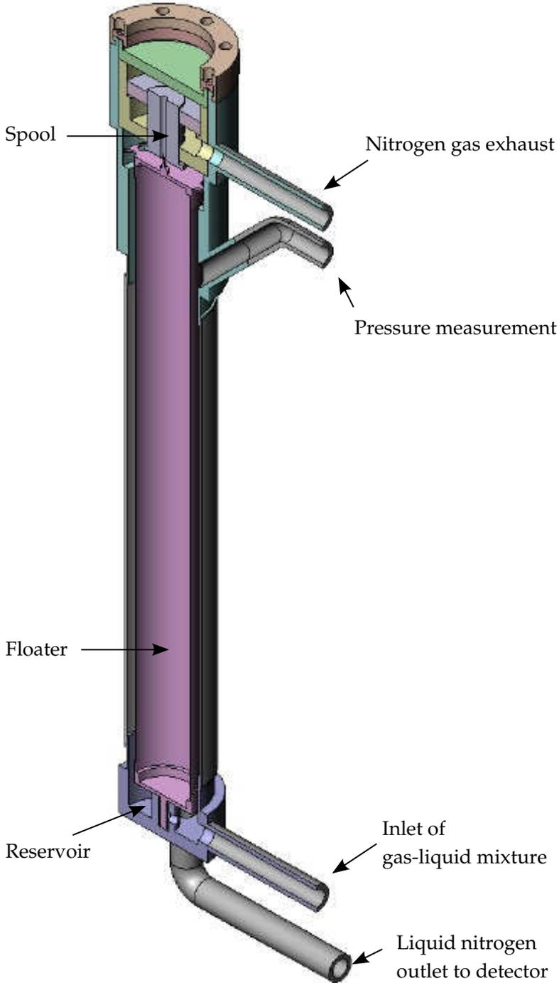
Figure 4.5: Cutaway view drawing of the phase separator.
