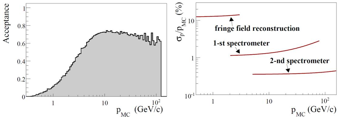
**Figure 2.4:** Reconstruction performance for charged tracks at COMPASS. Dependent on the particle momentum, the acceptance of the apparatus (left) and the momentum resolution for tracks reconstructed in the different spectrometer regions (right) are shown, from [COM07e].
