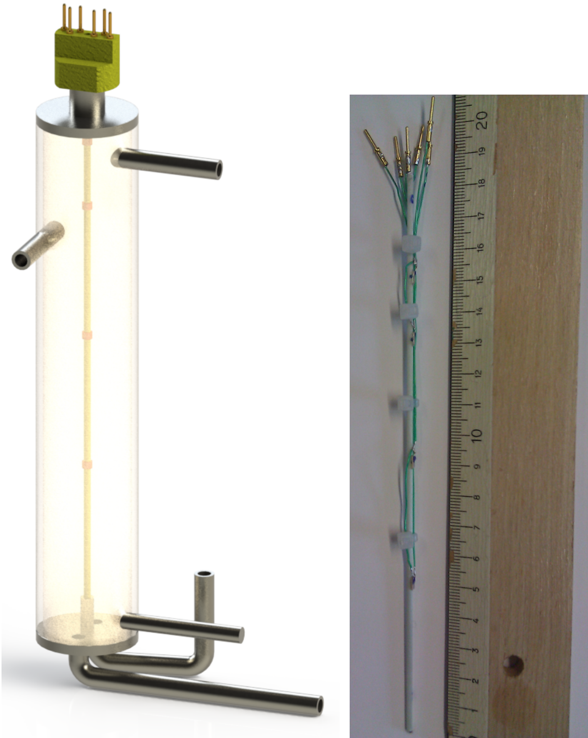
(a) Perspective CAD view of the modular phase separator (b) Close view of the rod carrying the Pt100 temperature sensors
