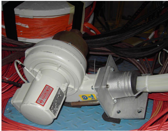
(a) Blower placed under the barrel
