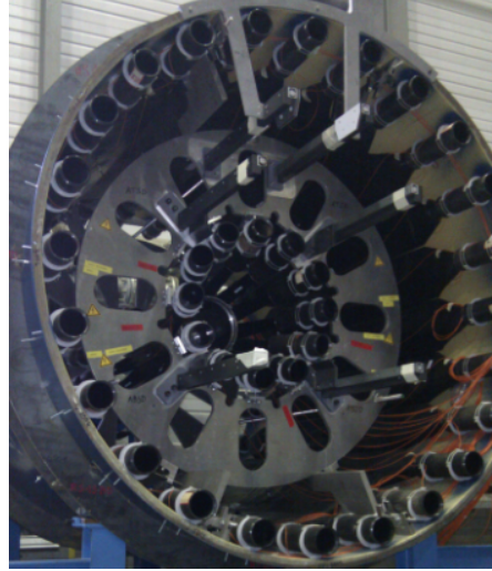
Figure 3.5: Photograph of the target vessel housing the Recoil Proton Detector, which is made of two scintillator barrels.
