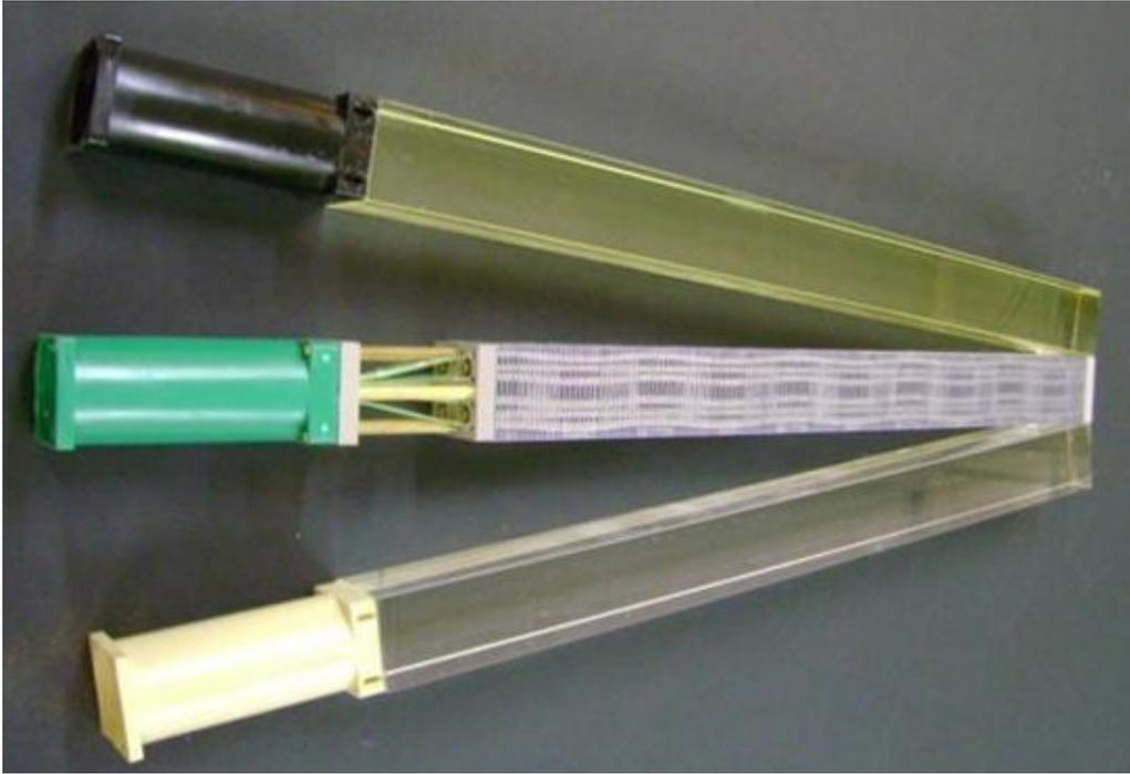
**Figure 2.7:** All three types of detector cells used in ECAL2.
