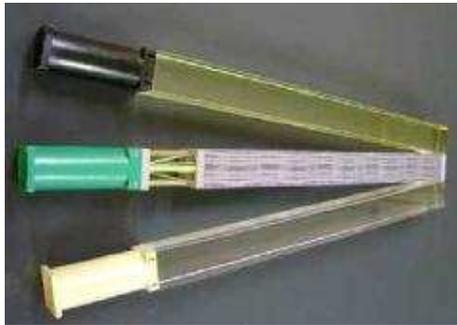
Figure 22: Different lead glass types for ECAL1 and ECAL2: upper and lower module. The central one is a SHASHLIK module [19].
