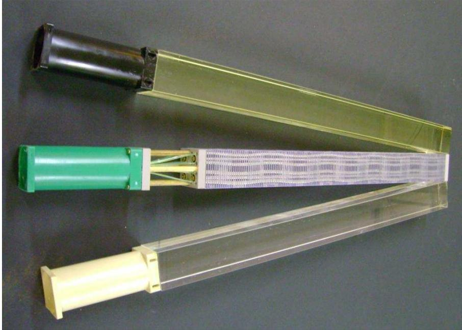
**Figure 5.** The 3 types of lead glass blocks used at COMPASS: radiation hard GAMS (top), shashlik (middle) and “normal” GAMS (bottom)
