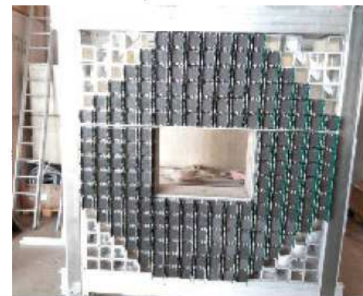
ECAL0 Calorimeter Shashlyk modules + MAPD readout ~ 2 × 2 m 2 , ~2200 ch.
