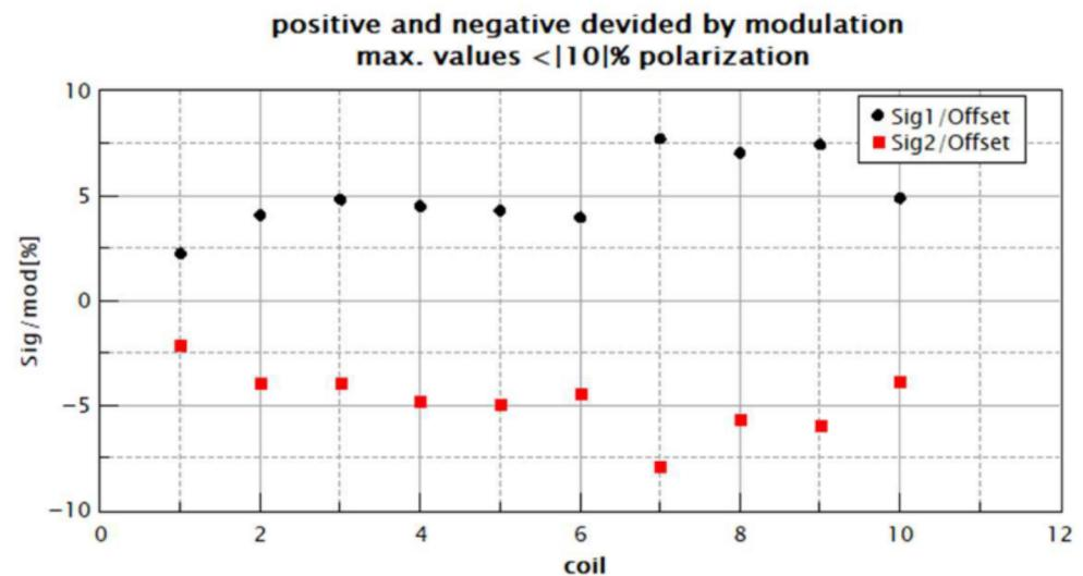
Uncertainties caused by modulation distortion less than 0.5%
