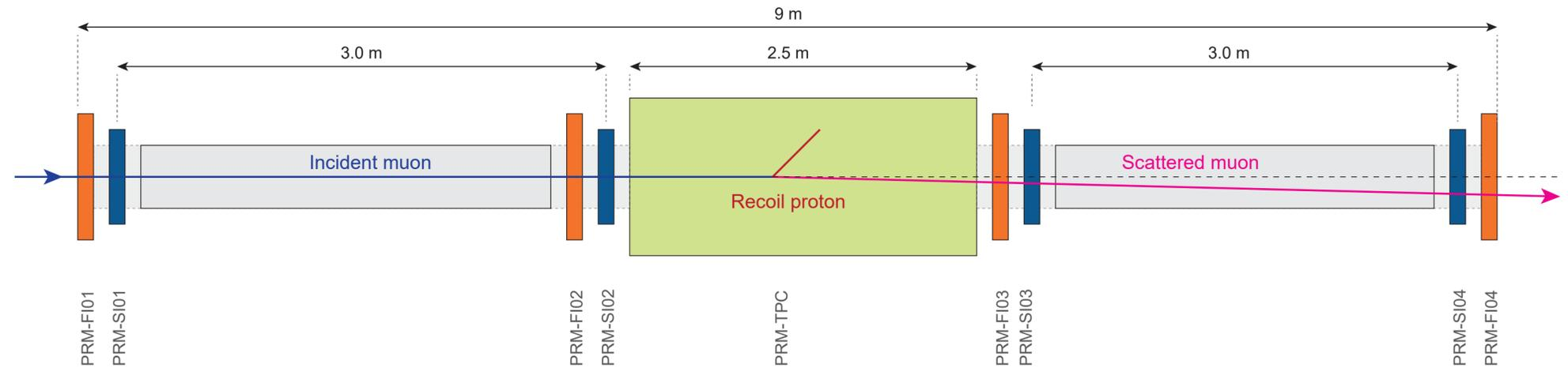
Legend: Scintillating-fiber hodoscope (orange), Silicon-pixel detector (blue), High-pressure hydrogen time-projection chamber (green), Helium-filled beam pipe (grey).
