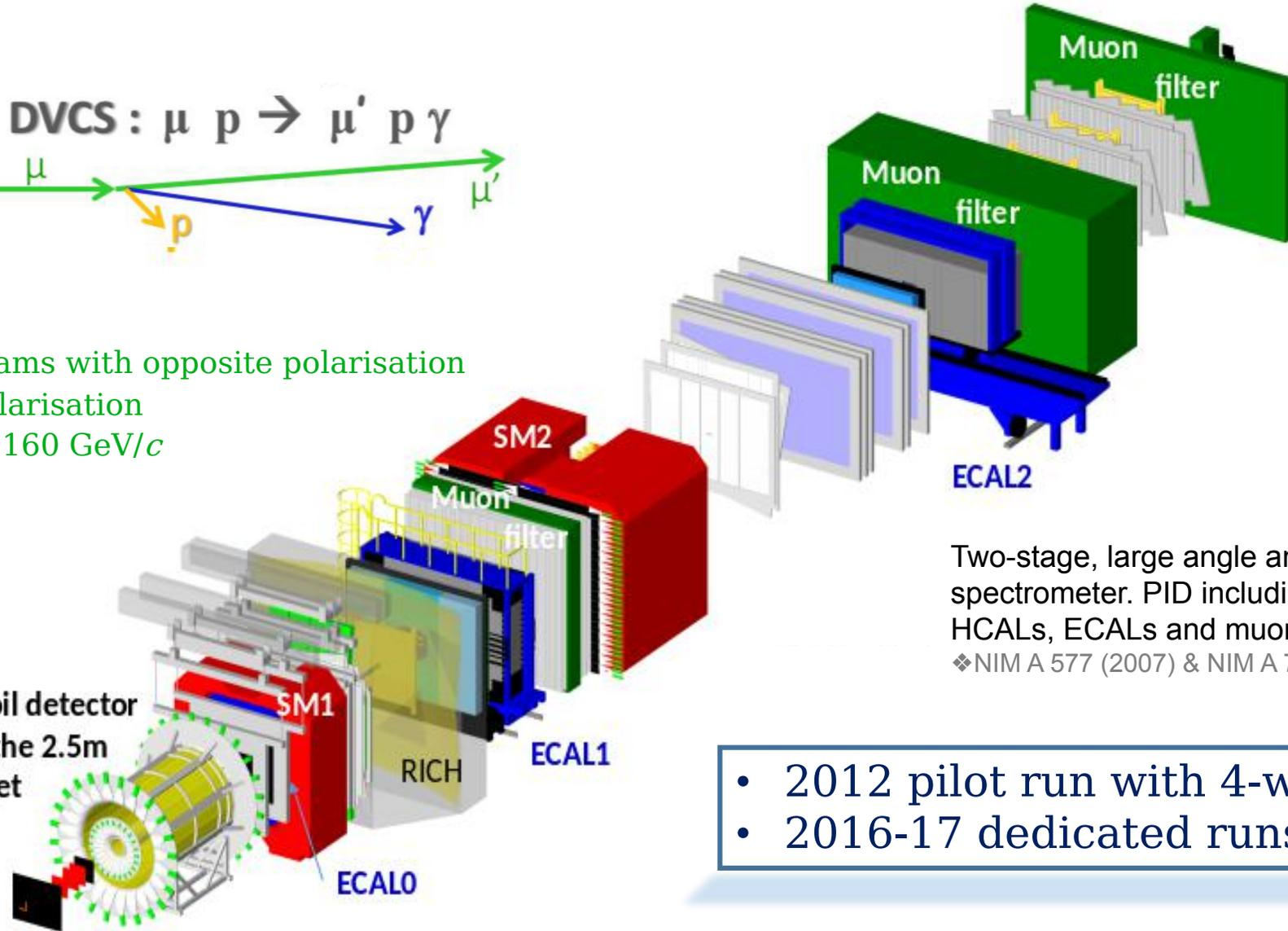
Two-stage, large angle and wide momentum range spectrometer. PID including hadron absorbers, RICH, HCALs, ECALs and muon filters.
