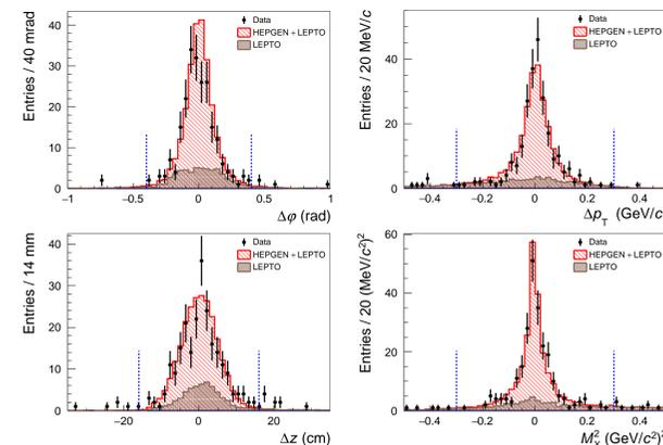
Distributions of the exclusivity variables:  $\Delta p_T$  and  $\Delta\phi$  in the upper row, and  $\Delta z$  and the four-momentum balance in the lower row [4, 9].
