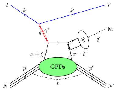
Handbag diagram of HEMP process  $lN \rightarrow l'N'M$ , where  $k$  ( $k'$ ) denotes the four-momentum of the scattering lepton,  $q$  is the four-momentum of the virtual photon  $\gamma^*$ ,  $p$  ( $p'$ ) represents the four-momentum of the target (recoiled) nucleon  $N$  ( $N'$ ), and  $M$  is the produced meson [4].
