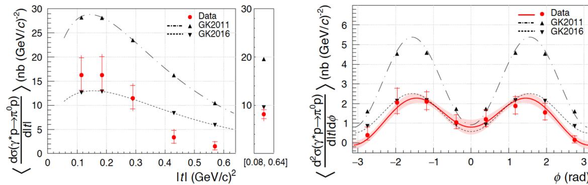
**Left:** The  $|t|$ -dependent differential exclusive  $\pi^0$  cross section after the integration over  $\phi$ . **Right:** The  $\phi$ -dependent exclusive  $\pi^0$  cross-section averaged over the measured  $|t|$  range. The black dash-dotted line denotes the earlier Goloskokov-Kroll parametrisation [8], the dashed line represents the later version of the GK model adjusted to the new results from [9].
