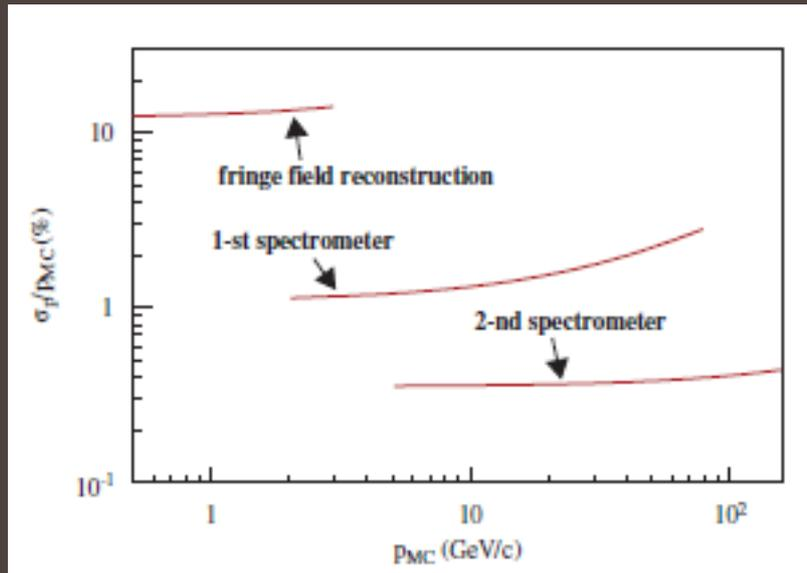
The relative error  $\sigma_p/p$  is about 0.5% for tracks reconstructed in both spectrometers ( $p \geq 5$  GeV/c) and about 1.2% for low momentum tracks reconstructed in the LAS only.
