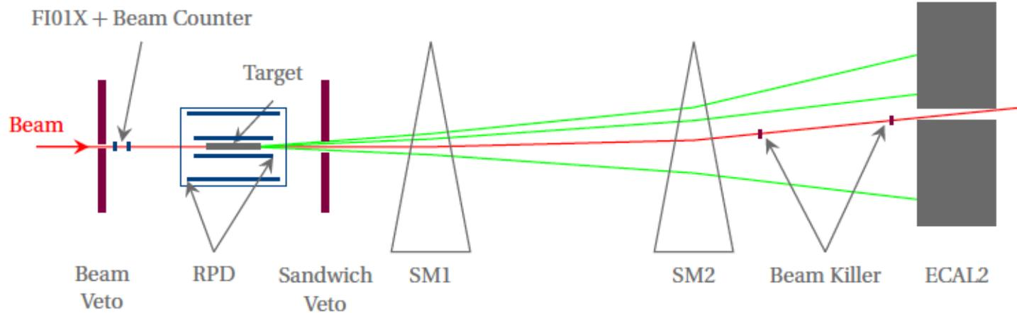
Figure 3.1: DT0 trigger scheme: Trigger (blue) and Veto (purple) components [59]. In the spectrometer, a non-interacting beam track (red) and an event with three charged tracks (green) is drawn for illustration.
