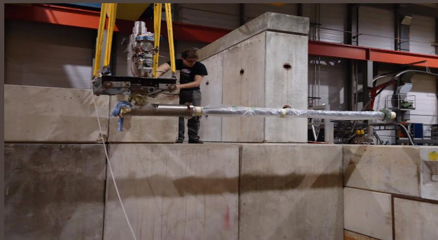
Liquid He target will be based on the existing liquid LH2 target
