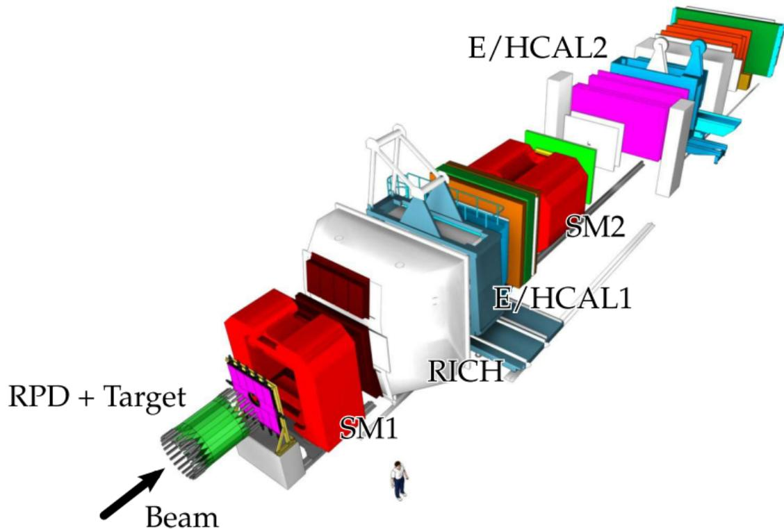
190 GeV/c<sup>2</sup> negative hadron (pion) beam on liquid hydrogen (proton) target.
