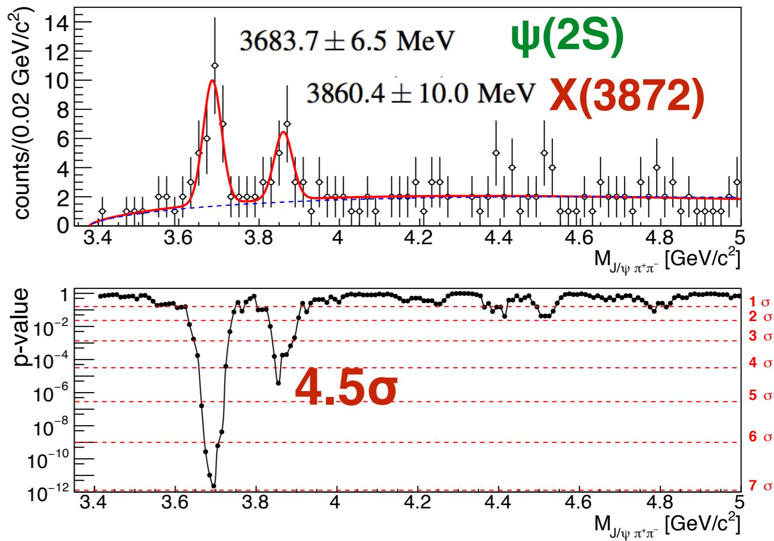
$$f(m) = Gaus(N_{\psi(2S)}, M_{\psi(2S)}, \sigma_M) + Gaus(N_{X(3872)}, M_{X(3872)}, \sigma_M) + c_1(m - m_0)^{c_2} e^{-c_3 m}.$$
