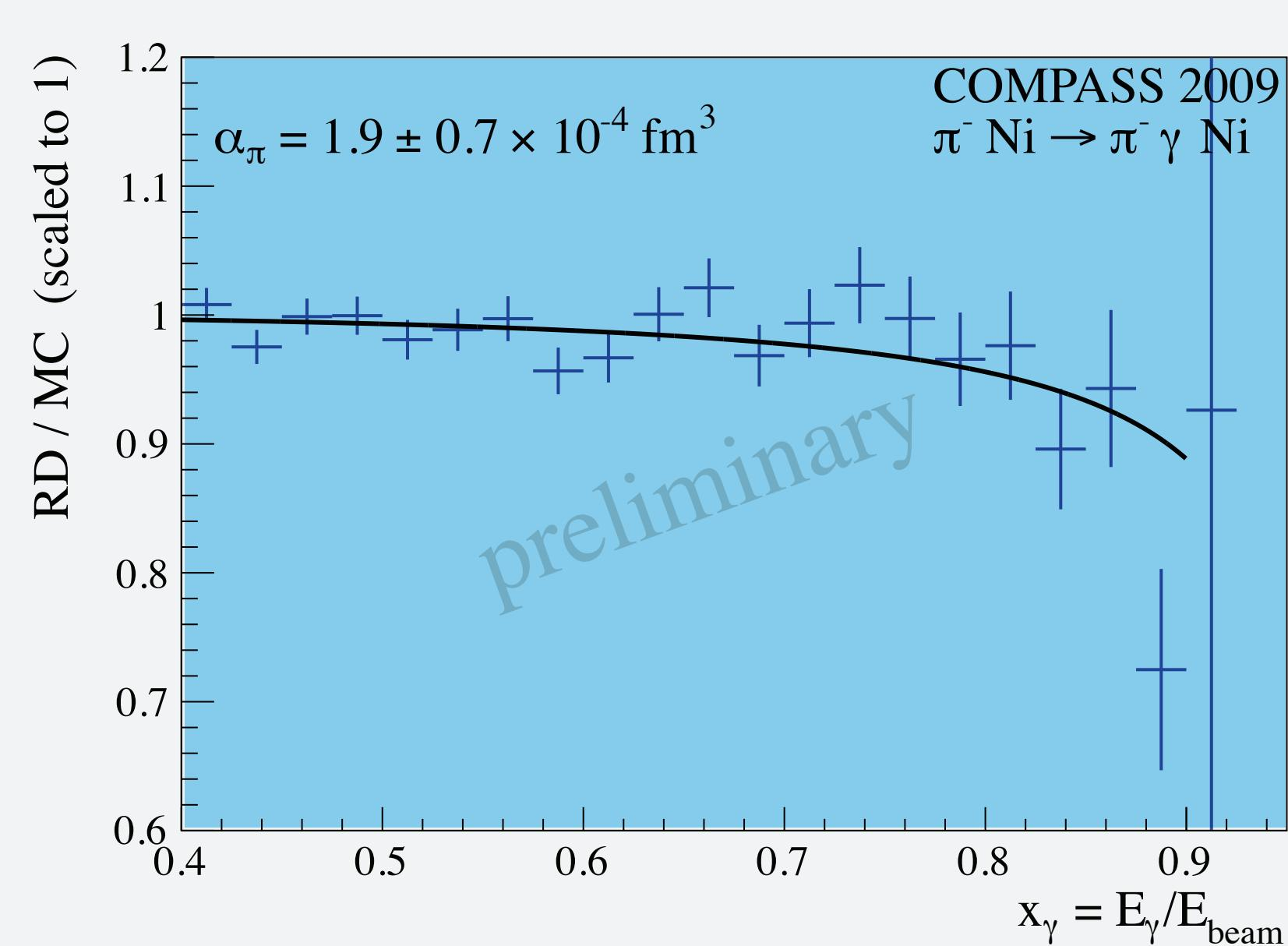
Polarizability fit to the  $x_\gamma$  distribution of the ratio of real data (RD) to a Monte Carlo (MC) simulation with zero polarizabilities.
