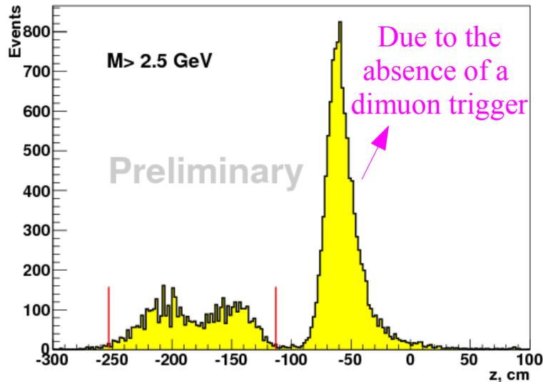
Reasonable  $Z_{\text{vertex}}$  separation, allowing to distinguish the 2 target cells and the absorber
