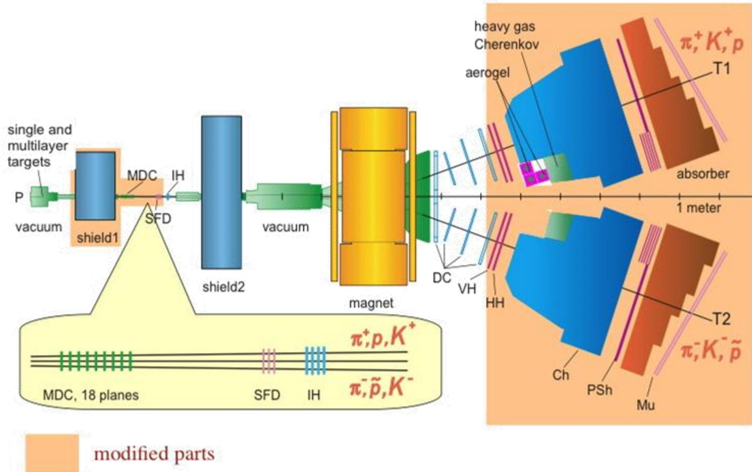
**MDC** - microdrift gas chambers, **SFD** - scintillating fiber detector, **IH** – ionization hodoscope. **DC** - drift chambers, **VH** – vertical hodoscopes, **HH** – horizontal hodoscopes, **Ch** – nitrogen Cherenkov, **PSh** - preshower detectors, **Mu** - muon detectors
