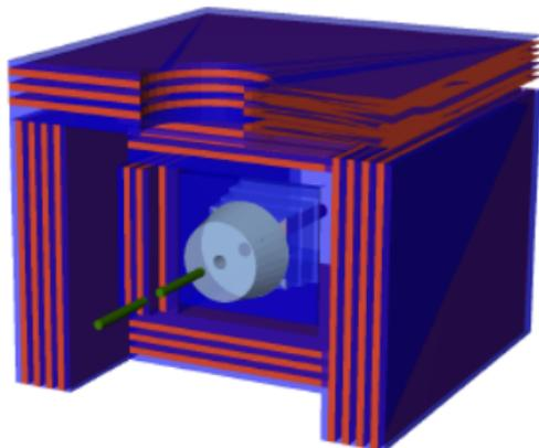
Structure of the absorber and its shielding
