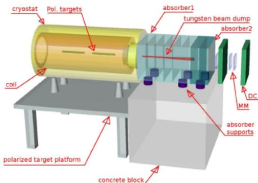
Possible setup of the target and absorber
