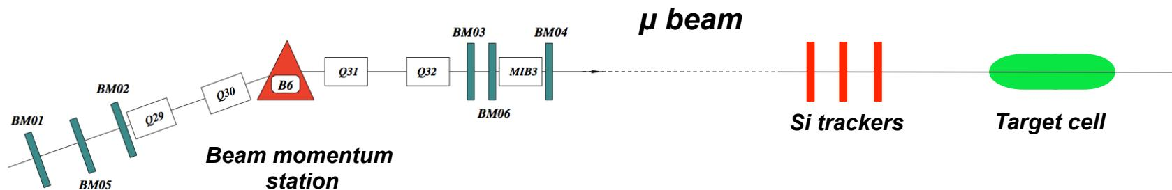
$$\sigma \propto \frac{N_{evts}}{Lumi \cdot Acceptance} \quad ; \quad L = \Phi_{beam} N_{target} \quad ; \quad \Phi_{beam} = \frac{N_{beam\ tracks}}{\Delta t N_{random}}$$
