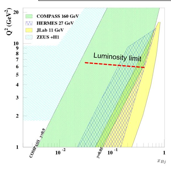
with a 2.5m long LH<sub>2</sub> target  $L = 10^{32} \text{ cm}^{-2} \text{ s}^{-1}$
