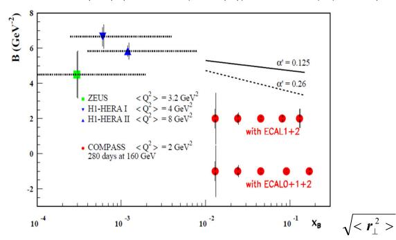
Projections: B accuracy ~0.1 GeV<sup>-2</sup> accuracy of  $\alpha$ ' ~3 $\sigma$  if  $\alpha$ '>0.16
