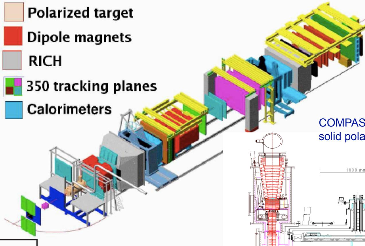
COMPASS  $\text{NH}_3$  or  ${}^6\text{LiD}$  solid polarised target
