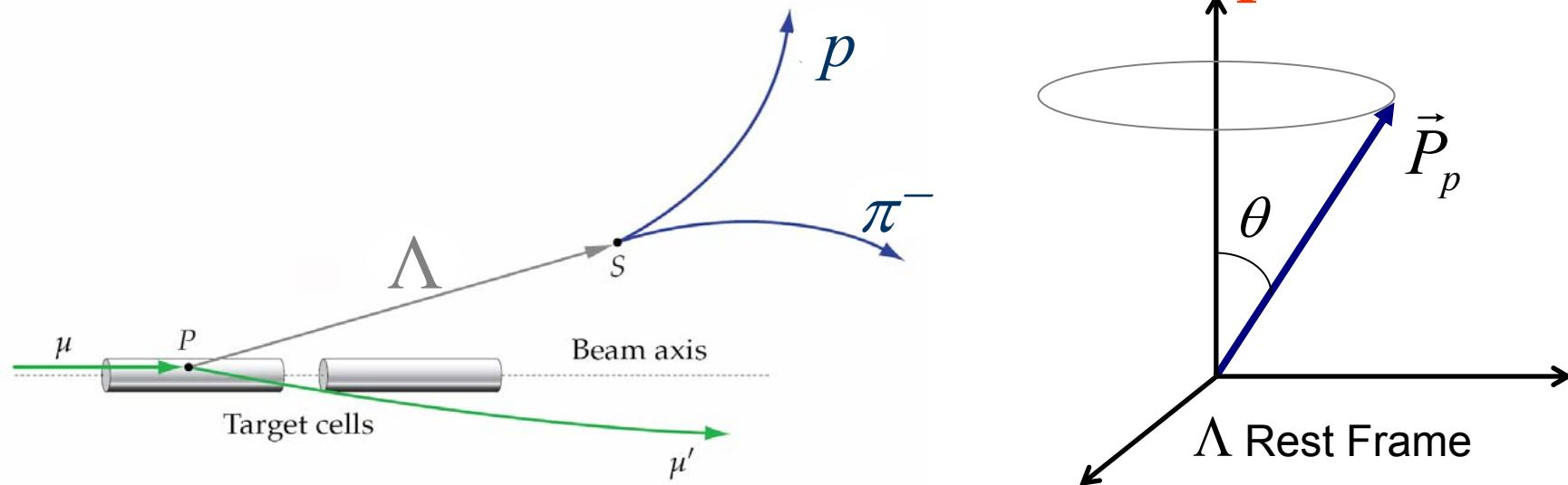
$\Lambda$  polarization  $P^\Lambda$  with respect to spin analyzer  $T'$  reveal itself in the angular distribution of decay proton :
