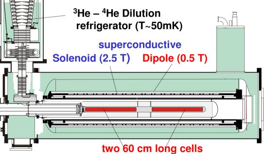
2002-2004: <sup>6</sup>LiD dilution factor f = 0.38 polarization P<sub>T</sub> = 50% ~20% of the time transversely polarised
