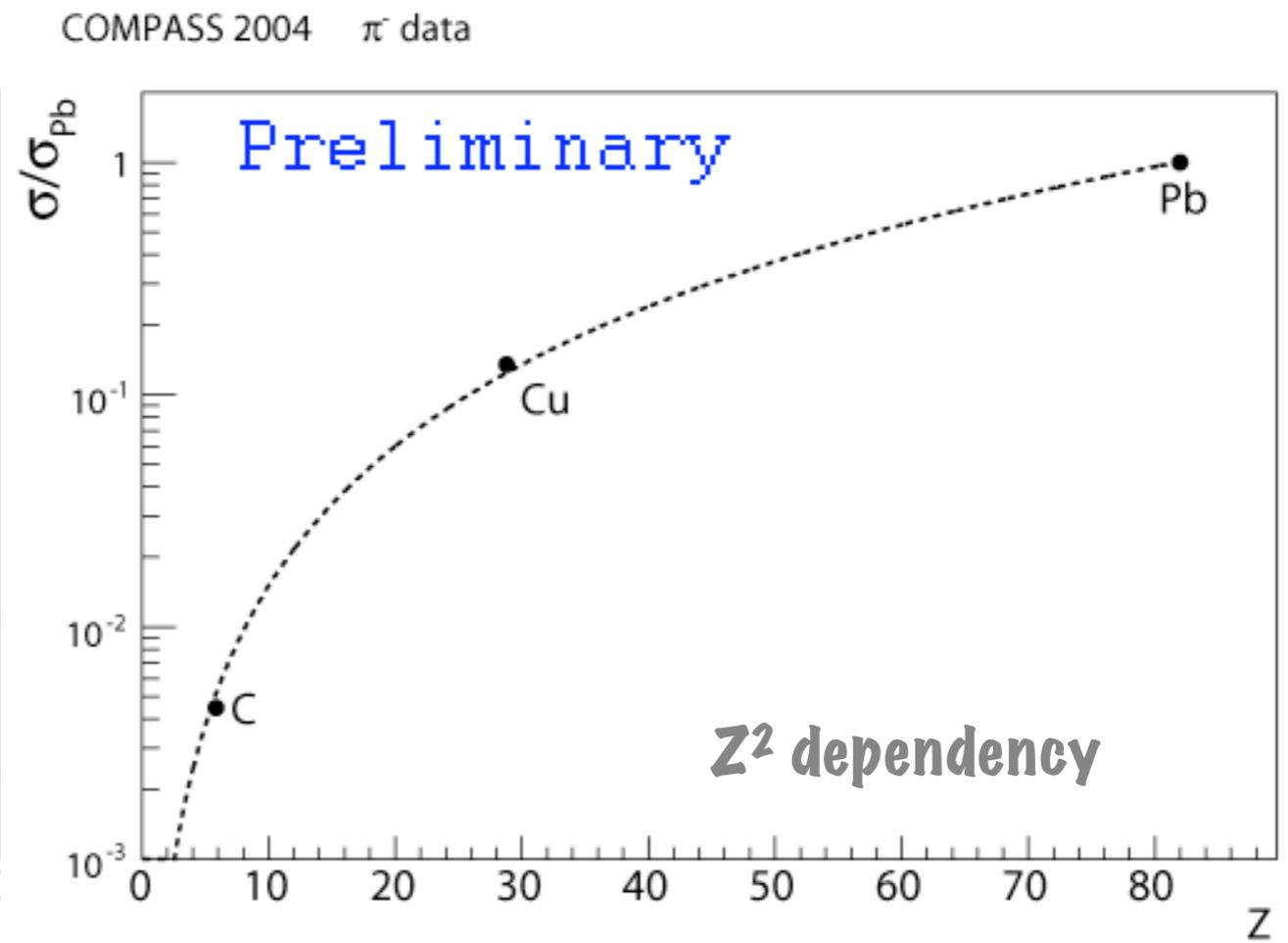
Strong dependency of Primakoff signal ( $Q=0$ ) to diffractive background ( $Q \gg 0.01$ ) ratio on the target material
