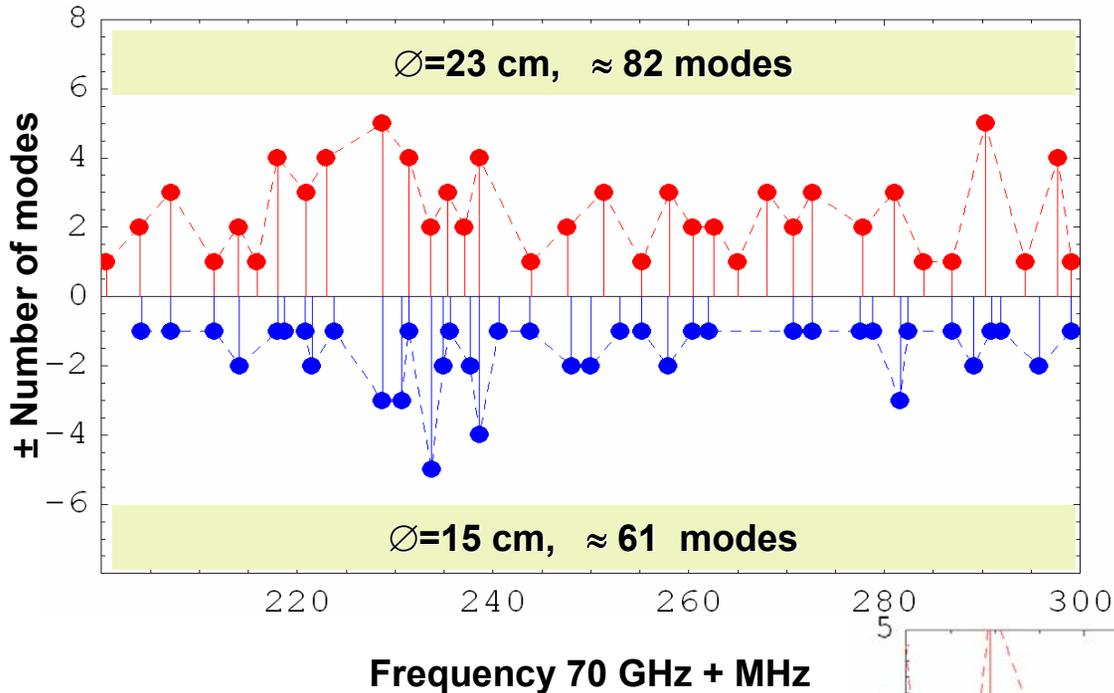
Result of the calculation for cylindrical cavity of different diameter:
