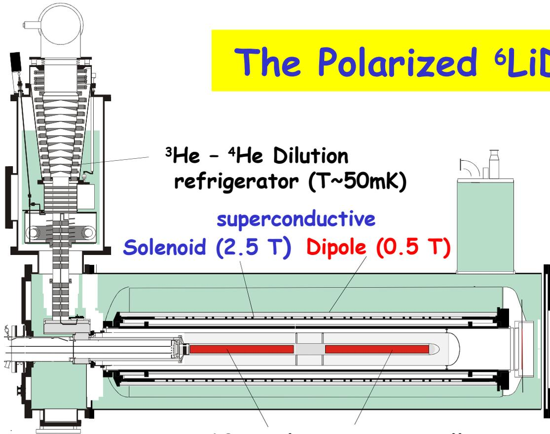
${}^3\text{He}$  -  ${}^4\text{He}$  Dilution refrigerator ( $T \sim 50\text{mK}$ )
