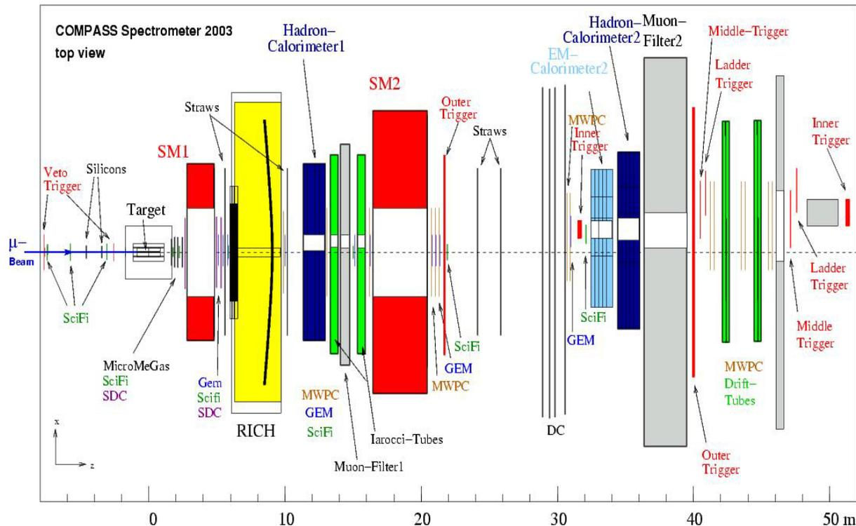
Double arm spectrometer, each with own magnet (SM1 and SM2), various trackers and PID for muons, electrons and hadrons
