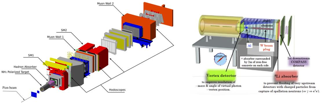
**Figure 3.** Left: sketch of the COMPASS setup for data taking with pion beam. Right: the ammonia target region.
