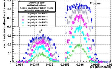
**Figure 2.** Separation of  $p$  and  $\pi^+$  beam particles in CEDAR detectors
