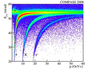
**Figure 3.** Cherenkov angle  $\theta_{Ch}$  vs. particle momentum in RICH detector
