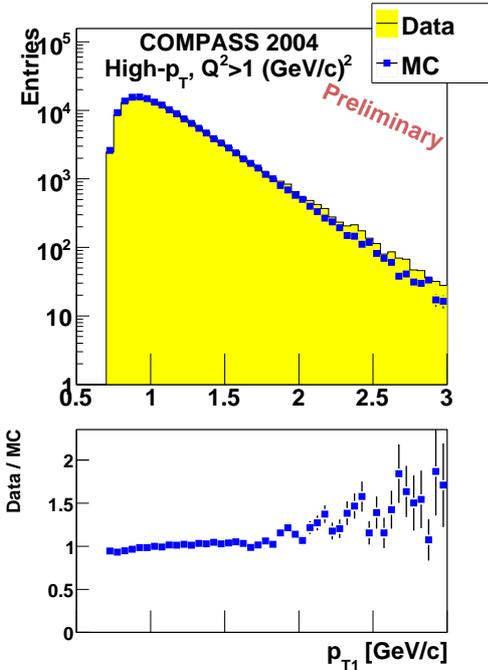
Figure 2. Data/MC comparison of the transverse momentum of the hadron with the largest  $p_T$ .
