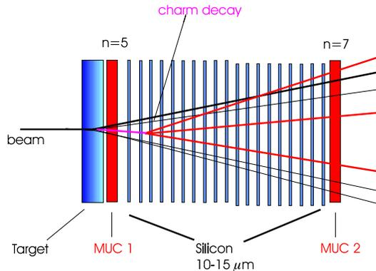
Fig. 3: Charm decay detector. 16–20 planes are spaced by 2 mm and have a pitch of 10–15  $\mu\text{m}$ .
