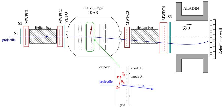
Figure 20: Example for the use of a high pressure active target TPC [56]
