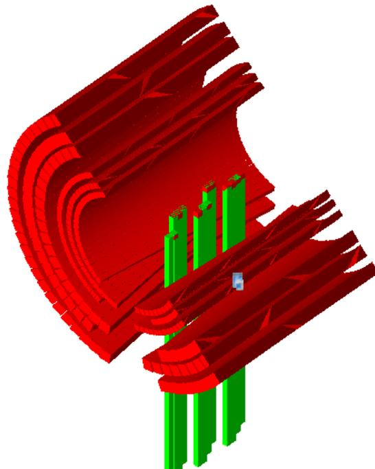
Figure 29: Layout of the active target made from scintillating fibres arranged along the beam direction.
