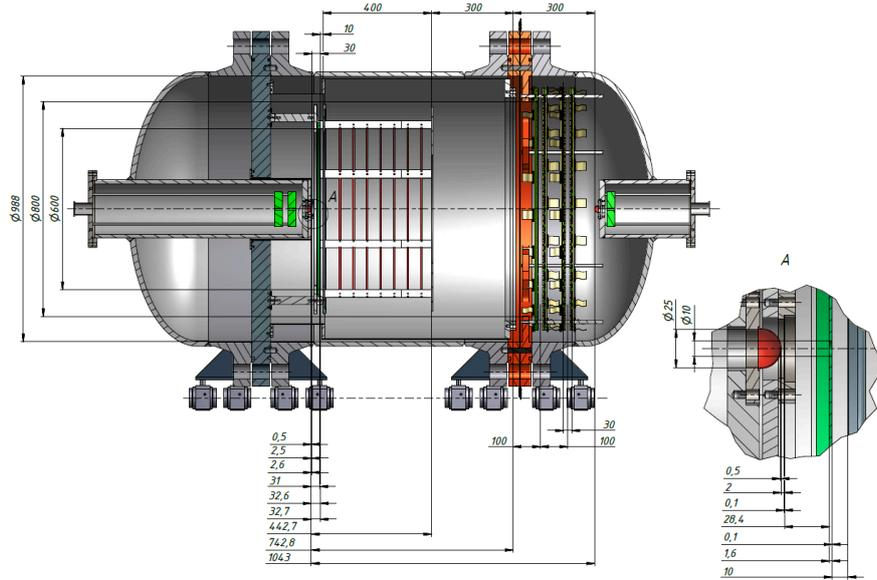
Figure 21: Sketch of the target TPC with pressure vessel as conceived for an elastic  $e^-p$  scattering experiment at MAMI. The forward tracker system on the right side of the vessel will not be installed for COMPASS.
