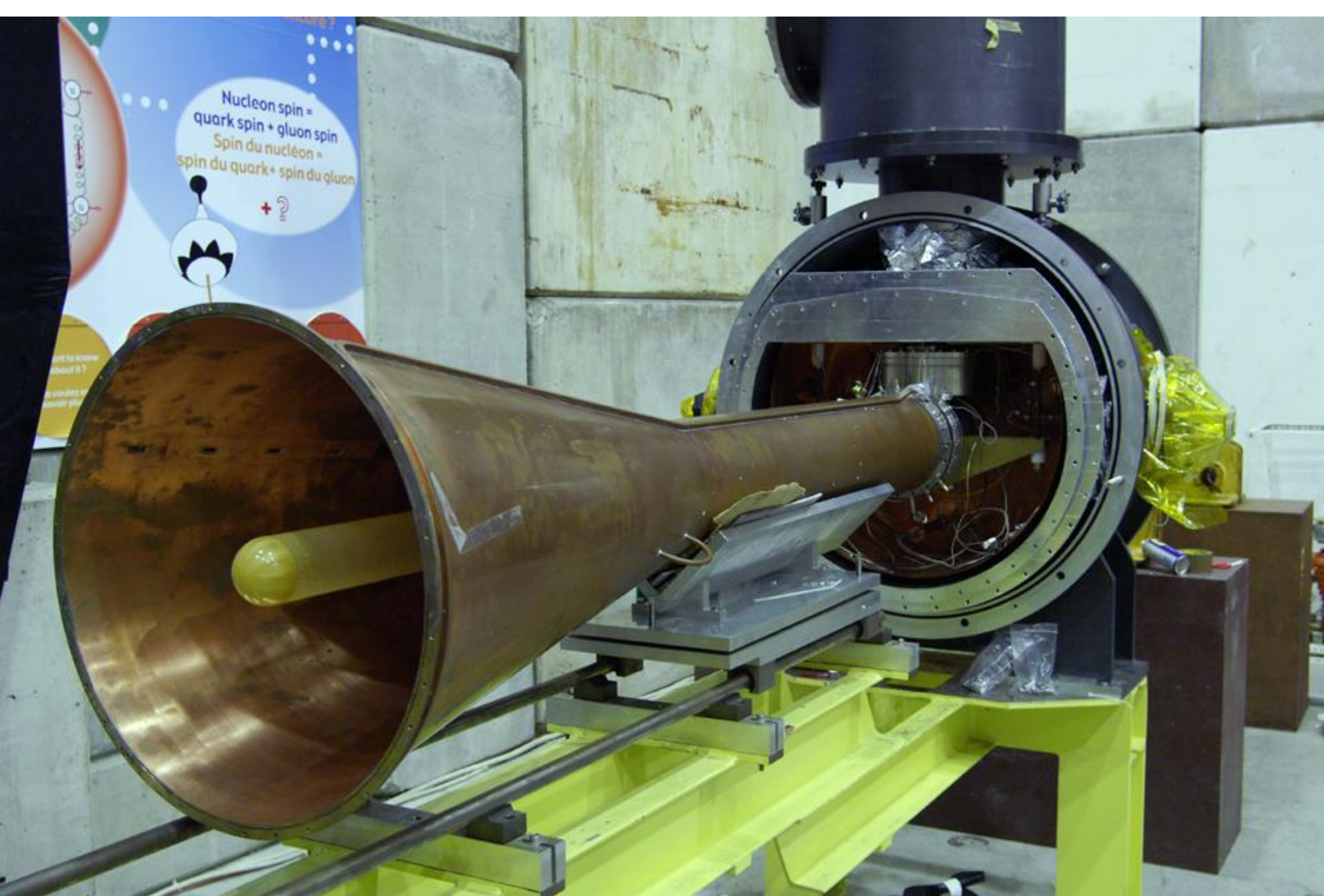
Insertion of the polarized target cells in the superconducting magnet
