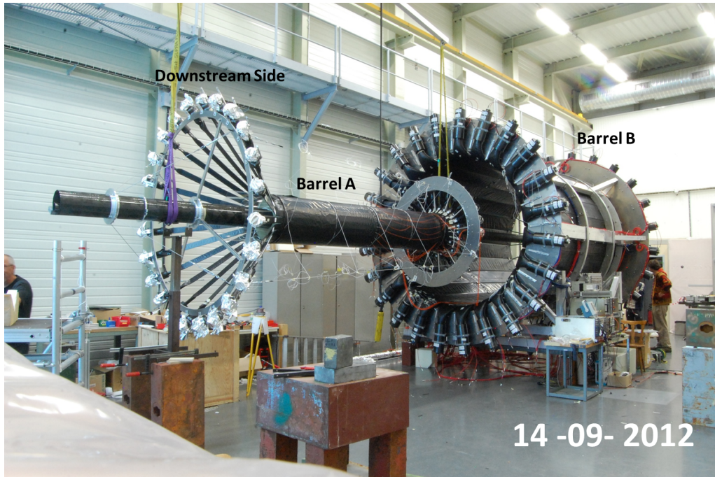
Figure 9: Picture taken on September 14, 2014, showing the insertion of the inner barrel A inside the outer barrel B of CAMERA. The long light guides on the downstream side of the inner barrel are visible on the left side of the picture.
