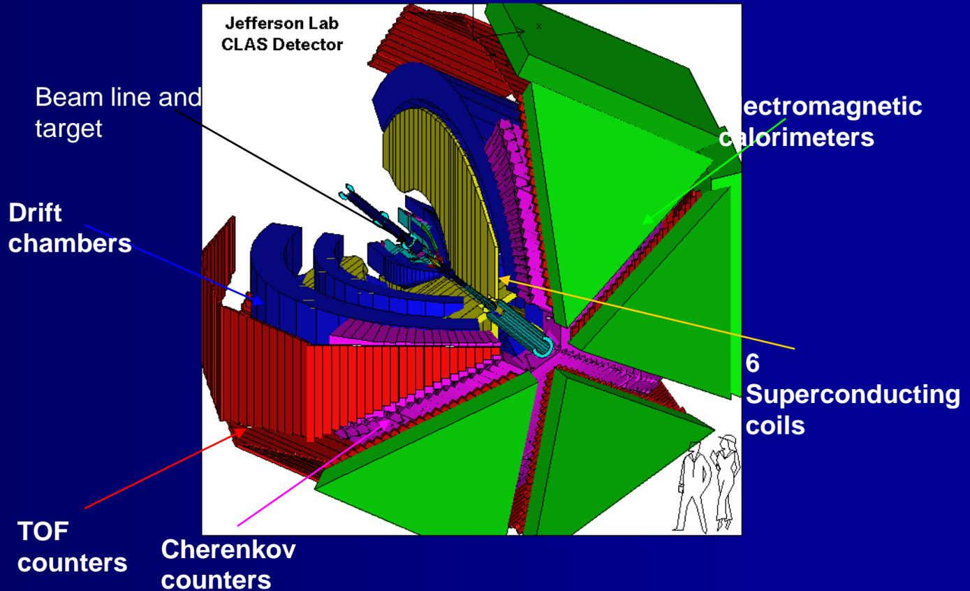
*CLAS* (forward carriage and side clamshells retracted)
