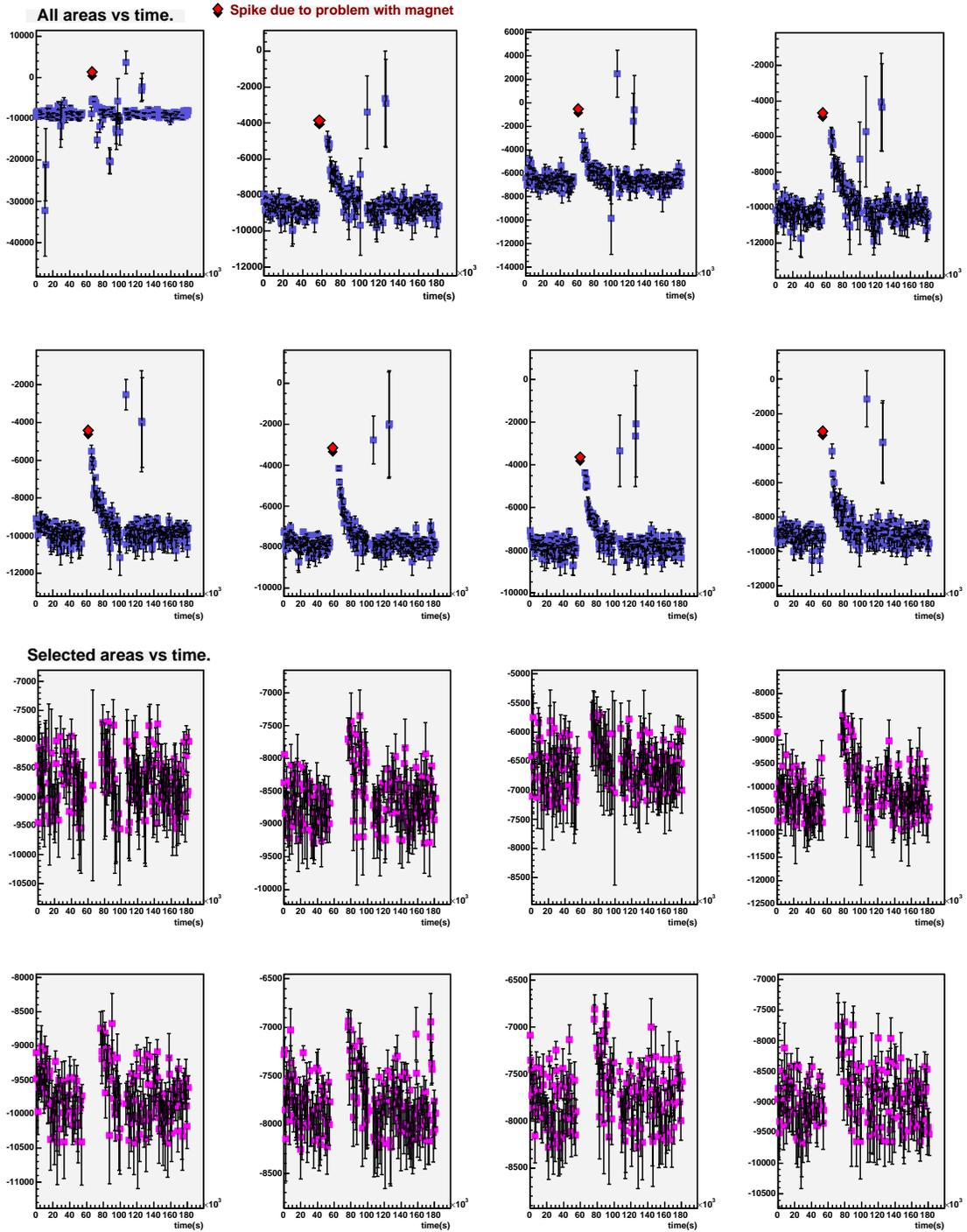
Figure 33: For the group of files TE2.1K. Note the spike due to a problem with the magnet. *Top*: plots of all the calculated TE areas against time for the 'Average method' in section 3.5. *Bottom*: selected areas against time. Each graph shows coil 1 to 4 at the top and coils 7 to 10 at the bottom.
