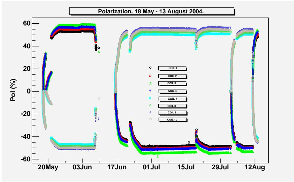
Figure 26: Polarization for each coil during the 2004 run: from 18 May to 13 August 2004. Upstream coils 1 to 4 are shown in black, red, green and blue, while downstream coils 7 to 10 are shown in turquoise, green, blue and grey.
