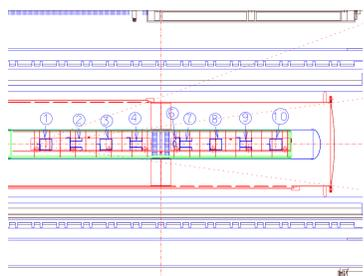
**Figure 1:** The microwave cavity with target cells inside superconducting magnet. The cells are inside glass fiber mixing chamber with liquid  $^3\text{He}/^4\text{He}$  mixture at 50 - 300 mK temperature. The NMR coils 1 - 4 are on the upstream target cell and 6 - 10 on the downstream cell. Two halves of the microwave cavity are separated with a microwave stopper [1]. Muon beam comes from left and produced particles in acceptance of 69 mrad come out from right.
