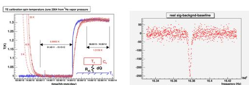
**Figure 6:** Left: Thermal equilibrium spin temperature during polarization calibration. The spin system (red) reaches thermal equilibrium with helium (blue) in about 15 hours. Primary thermometer based on  $^3\text{He}$  vapor pressure given by the International Temperature Scale ITS-90 is used. Right: Typical NMR signal during calibration.
