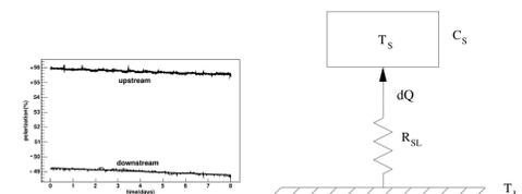
**Figure 9:** Polarization relaxation in frozen spin mode can be understood as heat flow to the nuclear spin system. At high polarization of 50 % the spin system with heat capacity  $C_s$  about 3 J/mol·K has spin temperature  $T_s$  around  $\pm 1$  mK.
