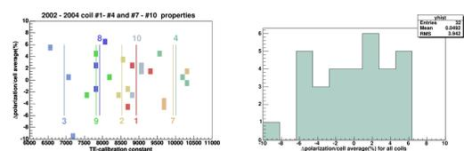
**Figure 8:** Left: Thermal equilibrium calibration constants vs. relative polarization of coils for 2002 - 2004. No correlation between coil position and polarization is seen. There is symmetry in the calibration constants with respect to the microwave stopper in center. Right: Histogram of relative coil polarizations 2001 - 2004. The deviation in the measured polarization seems to be less than relative 6 %.
