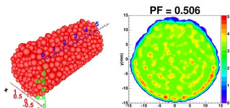
**Figure 3:** Simulated target material packing with 0.50 packing factor. The 6 cm long and 3 cm diameter cylinder is filled with 2 - 4 mm diameter spheres.
