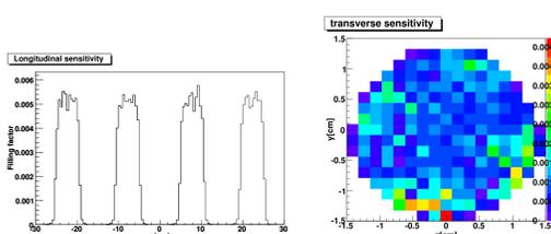
**Figure 4:** Left: NMR signal intensity along the beam axis for 2003 and 2004 upstream deuteron coils. The bin width is 0.5 cm. Summing the bins for each coil gives total filling factor of 0.05 - 0.06. Right: Transverse sensitivity from the 95 % signal volume for all upstream coils in 2003 and 2004. The bin size is about 0.18 cm  $\times$  0.18 cm. The sensitivity close to the coil on the surface of the target cell is some what better.
