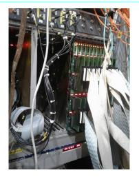
unplugging the unused TDC cards reduced the power consumption of the crate from 55A to
