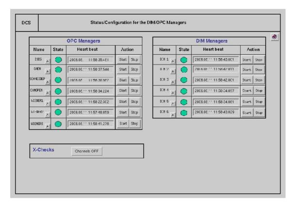
The DCS panel, accessible by clicking the "DCS" button on the left, shows the state of the servers used for monitoring/control of equipments (GREEN: running; RED: stopped). "Start/Stop" buttons can be used by the shift crew to restart managers that stopped for some reason.
