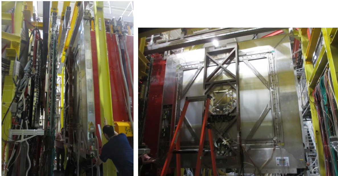
Attachment 6: The preparations for the installation of the DC05 detector. The detector DC04 is moved out to the garage position. Vertically across the center of the detector the GEM detector is placed (left picture).
