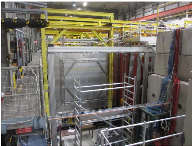
Attachment 7: The new DC05 detector (from [27]).
