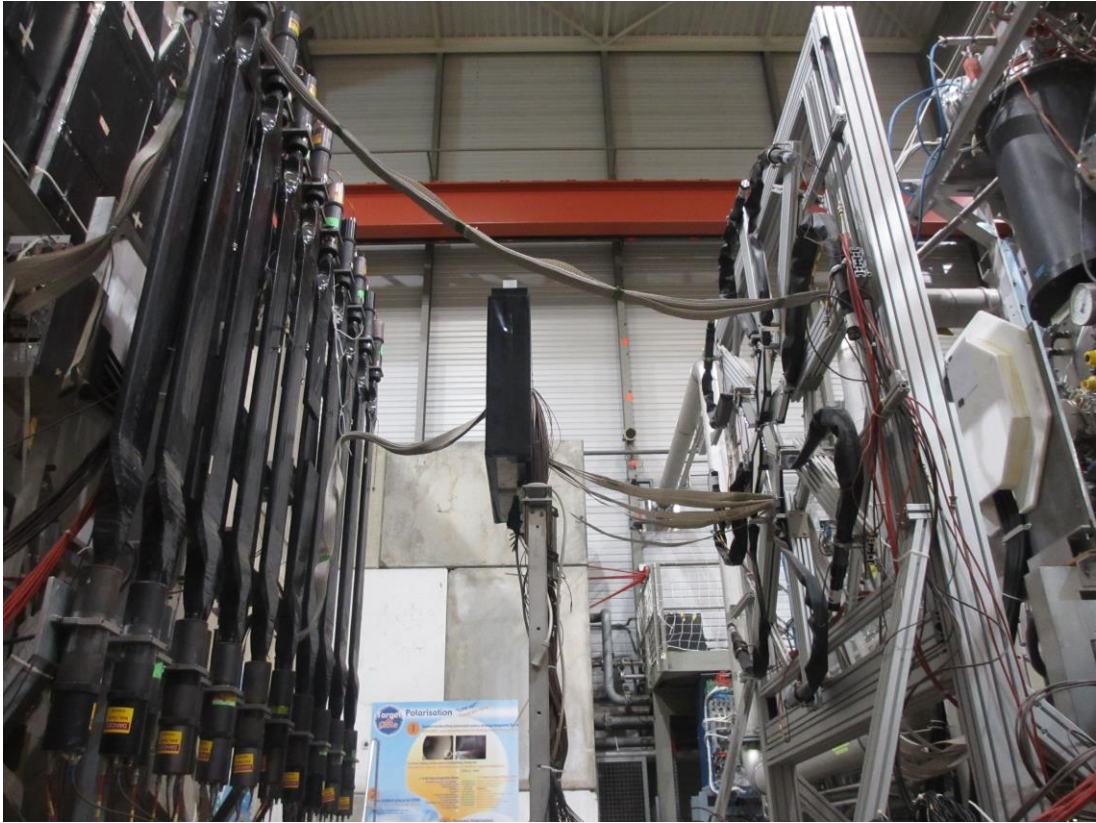
Attachment 5: The photograph of the beam telescope consisting of the VETOinner1 (first left), SciFi1.5 (middle), VETOinner2 (the next plane, on the right), and the SciFi3 (the very right).
