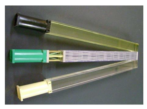
Figure 5. The 3 types of lead glass blocks used at COMPASS: radiation hard GAMS (top), shashlik (middle) and "normal" GAMS (bottom)
