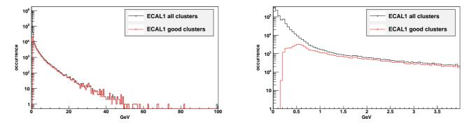
Figure 28. energy spectrum of clusters from ECAL1 (right) and a zoom into low energy area (left)
