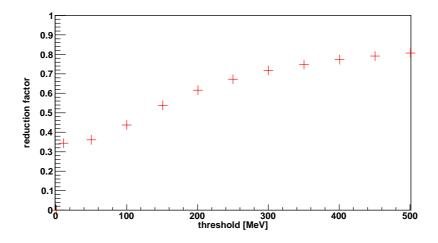
Figure 39. ECAL2 reduction factor of the bld algorithm at different thresholds
