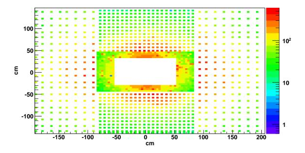
Figure 51. ECAL1 hitmap after applying bld and smd algorithms with the final thresholds
