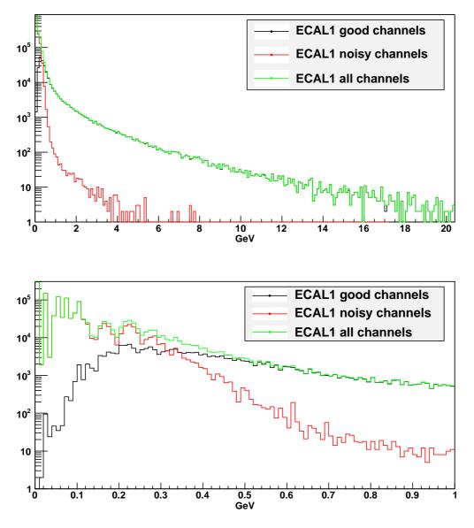
Figure 23. ECAL1 energy spectrum and zoom into low energy region
