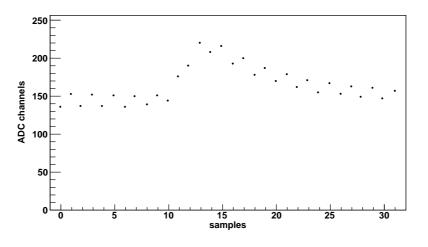
Figure 7. MSADC signal with uncorrected ADC baselines
