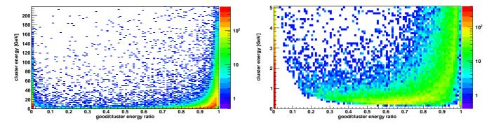
Figure 56. good/cluster energy plotted over cluster energy for ECAL1
