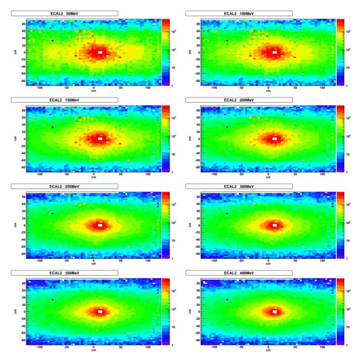
Figure 38. hitmaps for ECAL2 at different bld energy threshold
