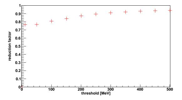
Figure 36. ECAL1 reduction factor of the bld algorithm at different thresholds
