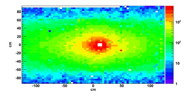
Figure 52. ECAL2 hitmap after applying bld and smd algorithms with the final thresholds
