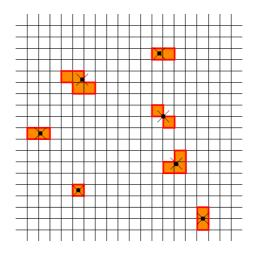
Figure 27. the "cluster" module is grouping all neighbouring cells together and calculating the centre of mass position
