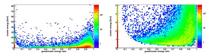
Figure 55. good/cluster energy plotted over cluster energy for ECAL1
