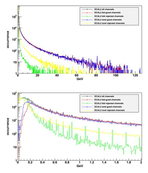
Figure 49. ECAL2 energy spectrum separated by algorithm
