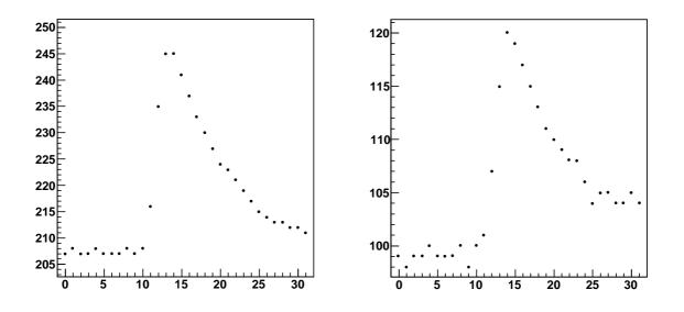
Figure 17. two signals from the SADC readout of ECAL2
