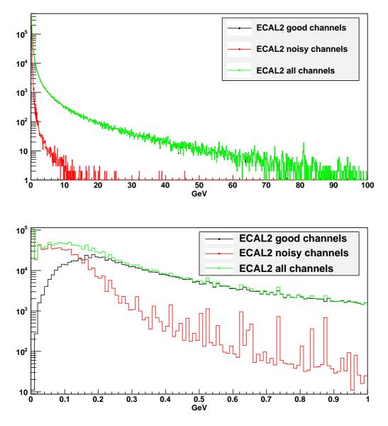
Figure 24. ECAL2 energy spectrum and zoom into low energy region
