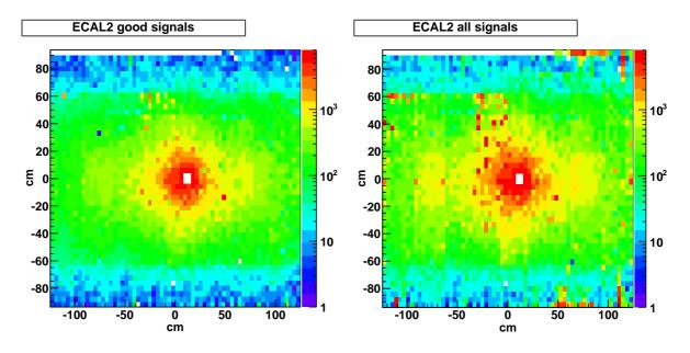
Figure 26. ECAL2 hitmaps for good (left) an all signals (right)
