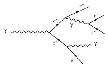
Figure 4. electromagnetic shower process
