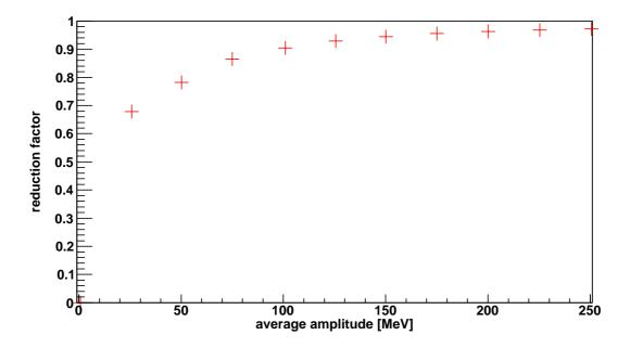
Figure 41. ECAL1 reduction factor of the smd algorithm at different thresholds
