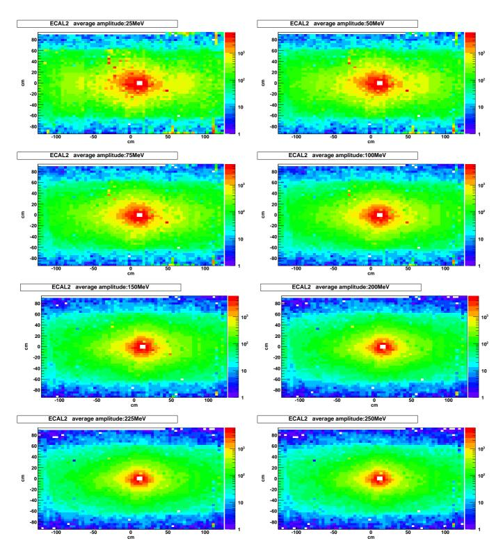
Figure 44. ECAL2 hitmaps for different average amplitudes
