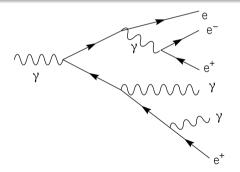
Figure: Schematic view of the start of an electromagnetic shower
